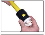
Stab pipe completely o into fitting so that the mark on the pipe is within 1/8" from the fitting entrance.
