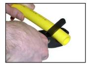
If using ID chamfer tool with gauge, check for proper chamfer by inserting pipe on gauge up to the o ring. With proper chamfer, o ring will begin to enter pipe.
